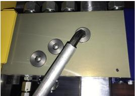
The replacements need a spanner 24 to tighten them. If available, a gear spanner 24 mm (ratchet spanner, gear wrench) does the best job.
