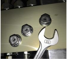
Use the spanner 24mm to tighten the plugs. Screw the plugs in as tight as possible (torque between 140 and as high as 180 Nm)
