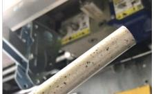
Shorten the short stem of the Allen key (as short as possible) and keep in mind that it still has to go into the hexagon socket of the plug (which is 11 mm deep). Shortening this stem will result in more room for your hand to be able to apply enough force to pull. The plug should be tightened with about 140 Nm or higher.
